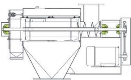
In addition to one motor-end bearing and one inboard bearing adjacent to the material infeed chute, three-bearing designs incorporate a bearing on the exterior of a hinged cover at the discharge end of the screener.
