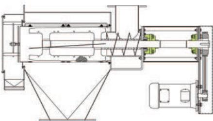
Two-bearing designs utilize one motor-end bearing, and one inboard bearing adjacent to the material infeed chute (no bearing on end cover).
