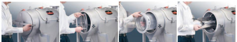
The hinged end cover is opened using quick-disconnect clamps, allowing the retaining plate, screen and paddle assembly to slide freely from the cantilevered shaft. Note: Two-bearing model shown requires no bearing on end cover.
