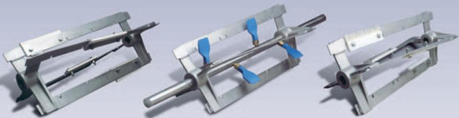
Rubber wiper blades handle fibrous material that would otherwise become entangled in brush bristles or wrap around serrated edges. Rubber blades allow oversize particles to pass by the rotating blade, and are also effective in liquid/solids separations.
