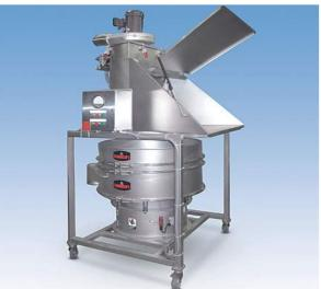
The Kason combination Bag Dump Screener/Dust Collector scalps bag scraps and other oversize materials from manually dumped bulk materials while protecting the operator and plant environment against dust contamination.
