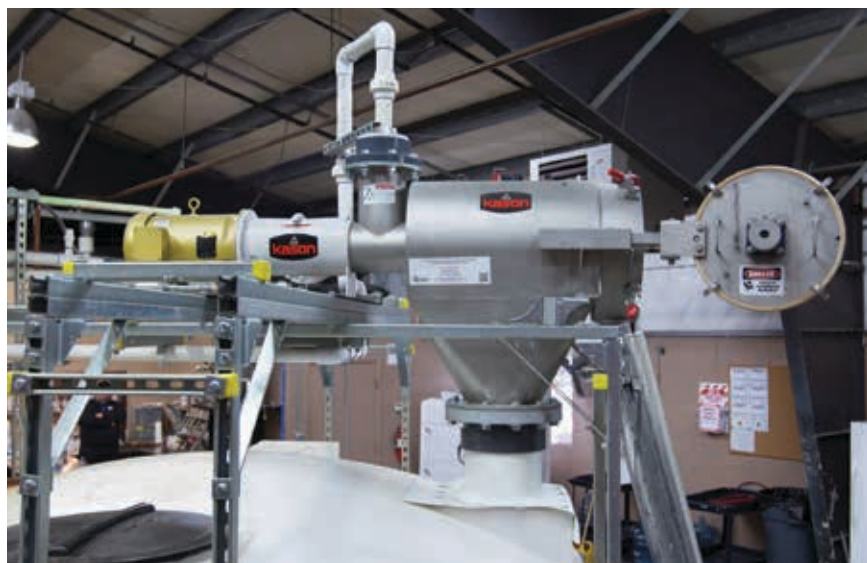
The sifter measures 1899mm in length including the 3hp (2.2kW) motor, and processes 189 litres of stillage per minute
