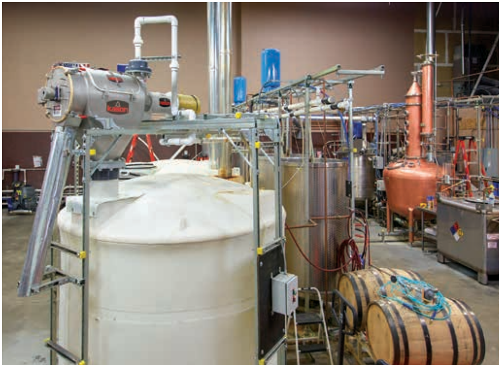
The Centri-Sifter centrifugal sifter separates about 3400 kg per week of fine grain particles from 8 Feathers stillage. The dewatered solids pass through the chute in foreground. The water gravity-discharges into the 7570L vat below
