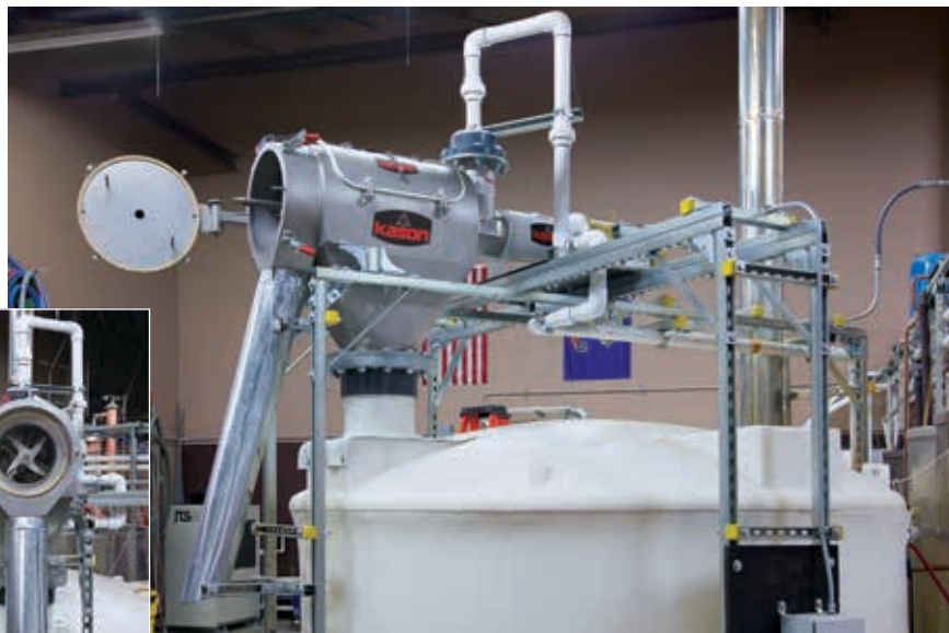
Opening the hinged end cover of the centrifugal separator allows the paddle assembly and screen cylinder to slide off the cantilevered shaft
