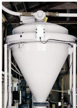
Scale hopper with Aeropass valve at top
