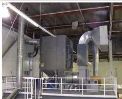
DustHog SFC 32-4 with Safety Filter used for blending powdered cheese, baking mixes and tortillas.
