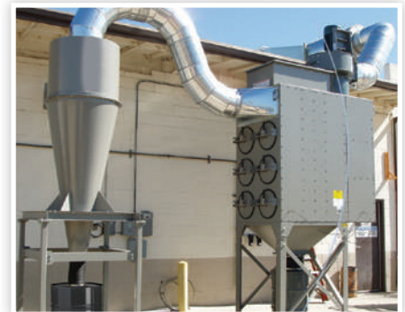
DustHog SFC 12-3 with Cyclone used for blending dry dairy and other food ingredients for baked goods and snack foods.
