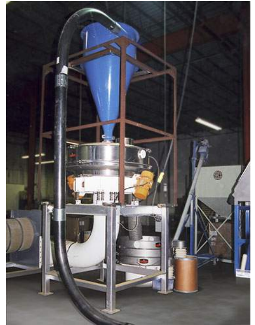
Cellulose-plastic pellets move from a pelletizer to a cyclone separator via pneumatic conveyor, and are gravity-discharged into a 60 in. (1525 mm) diameter circular vibratory cooler which reduces their temperature to 100°F (38°C) and moisture content to less than 1%. Pellets are classified into on-size, over-size and fines by a 48 in. (1225 mm) Kason VIBROSCREEN® circular vibratory separator.
