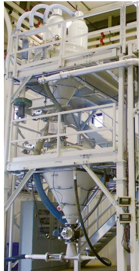
Photo 2 - Dense phase conveying system with rotary valve
