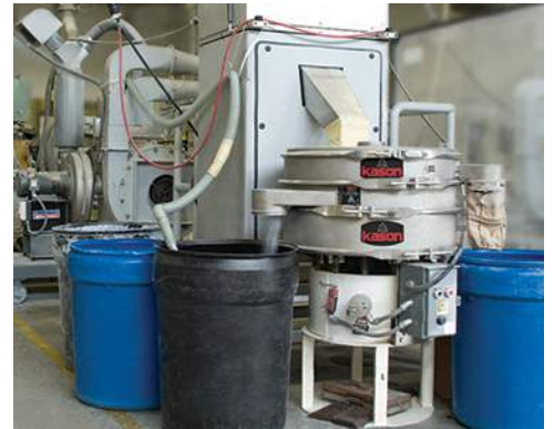
Kason circular VIBROSCREEN® pellet classifier with two screening decks was one of six specified for use at the end of pelletizing extruders to save floor space. Rotuba has six 24 in diameter (610 mm) classifiers, each replacing a 2 ft by 7 ft (61 cm by 213 cm) rectangular screening unit.
