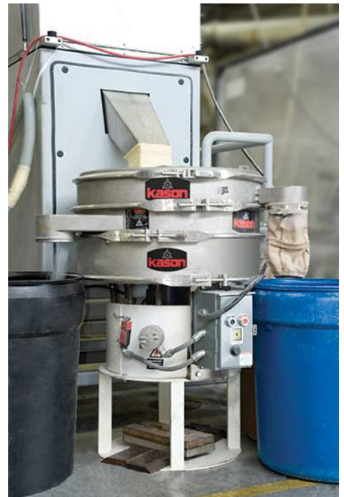
Oversize pellets are scalped by the upper deck of the vibratory screener, with undersize pellets and dust collected and discharged by a sloping lower pan. On-spec pellets are captured and discharged from the middle deck.
