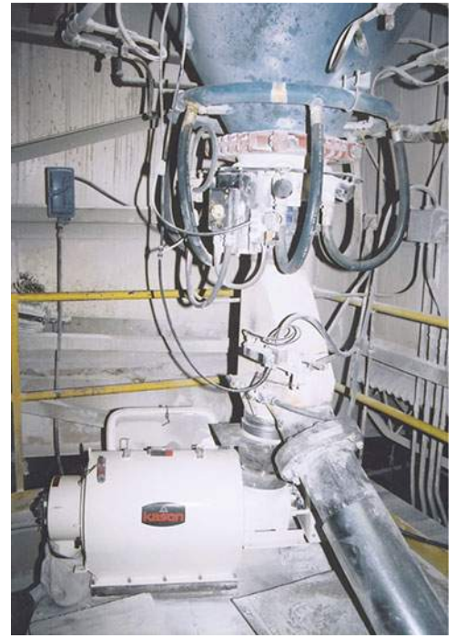
4000 lb (1814 kg) of sand-silica powder sprayed with liquid plasticizer in pneumatic blender is delumped in 12 minutes using a CENTRI-SIFTER centrifugal screener.
