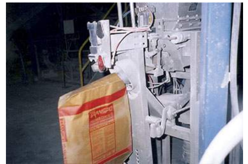
A 4000-lb (1814 kg) batch of polymer concrete is bagged in 15 minutes.
