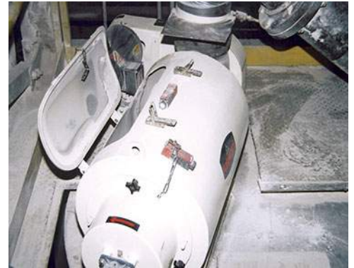
Small footprint of CENTRI-SIFTER centrifugal screener fits into tight space. Access door allows quick inspection, cleaning or screen changing. Slide gate valve (rear) controls flow rate of powder entering the screener from the blender.
