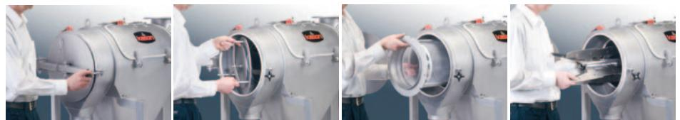
The hinged end cover is opened using quick-disconnect clamps, allowing the retaining plate, screen and paddle assembly to slide freely from the cantilevered shaft. Note: Two-bearing model shown requires no bearing on end cover.
