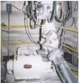
In 12 minutes, CENTRI-SIFTER™ screener sifts 4000 lb (1814 kg) of polymer concrete discharged from pneumatic blender, while eliminating previous screen blinding problem.
