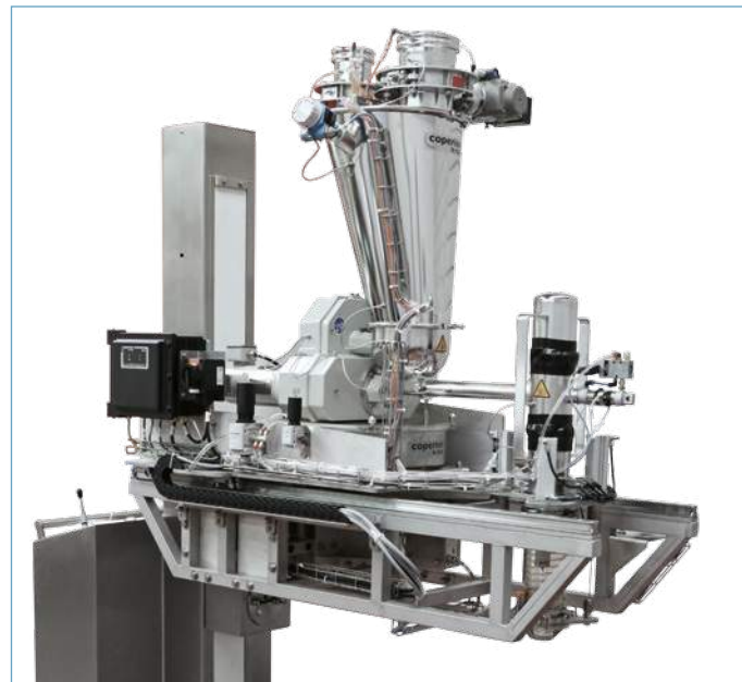
Photo 1 - Feeder on mobile lift system for maximum accessibility
