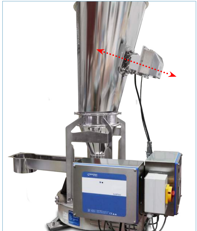
Photo 3: Vibratory feeder with ActiFlow smart bulk solid activator mounted at the back of the hopper and the control unit in the foreground.
