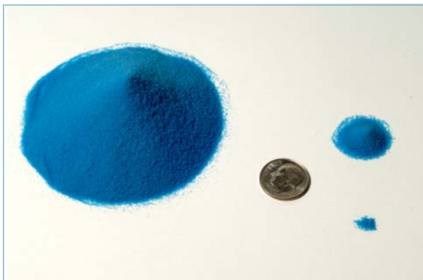
At a feed rate of 20g/hr, the three piles of material represent an hour's throughput (20g), a minute's discharge (0.33g) and second's dosing (0.005g). The dime shows physical scale.
