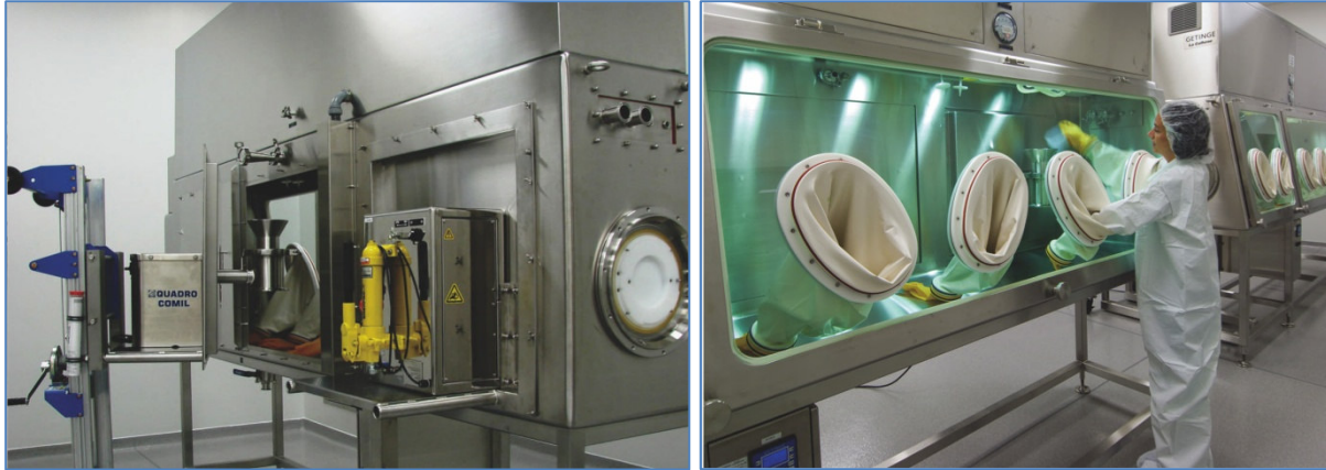
Quadro® Comil® U5 – “Through-The-Wall” Design incorporated into a Glove Box Isolator
