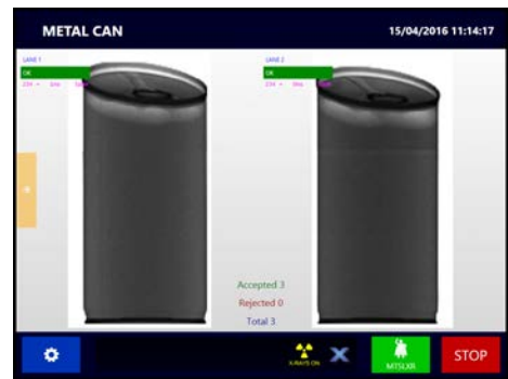
Figure 9: Product is inspected twice to catch any potential contaminants.
